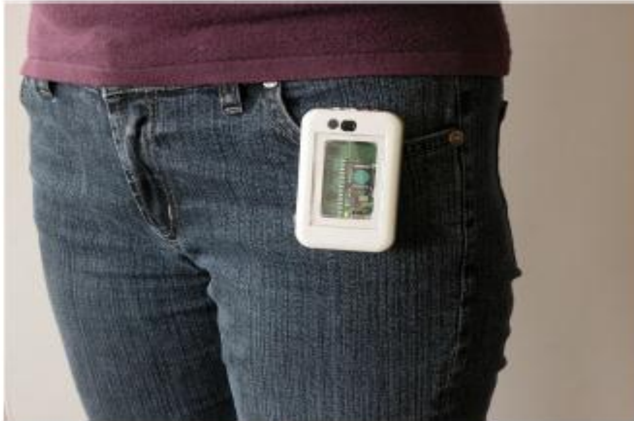
Figure 2 The custom-made belt-worn device incorporating accelerometer, microphone and light sensor.
